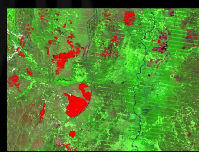
Figure 2: Landsat (30m) burned area maps offer increased sensitivity to small agricultural fires and reveal spatial patterns of burning in greater detail to global MODIS (500m) products.
