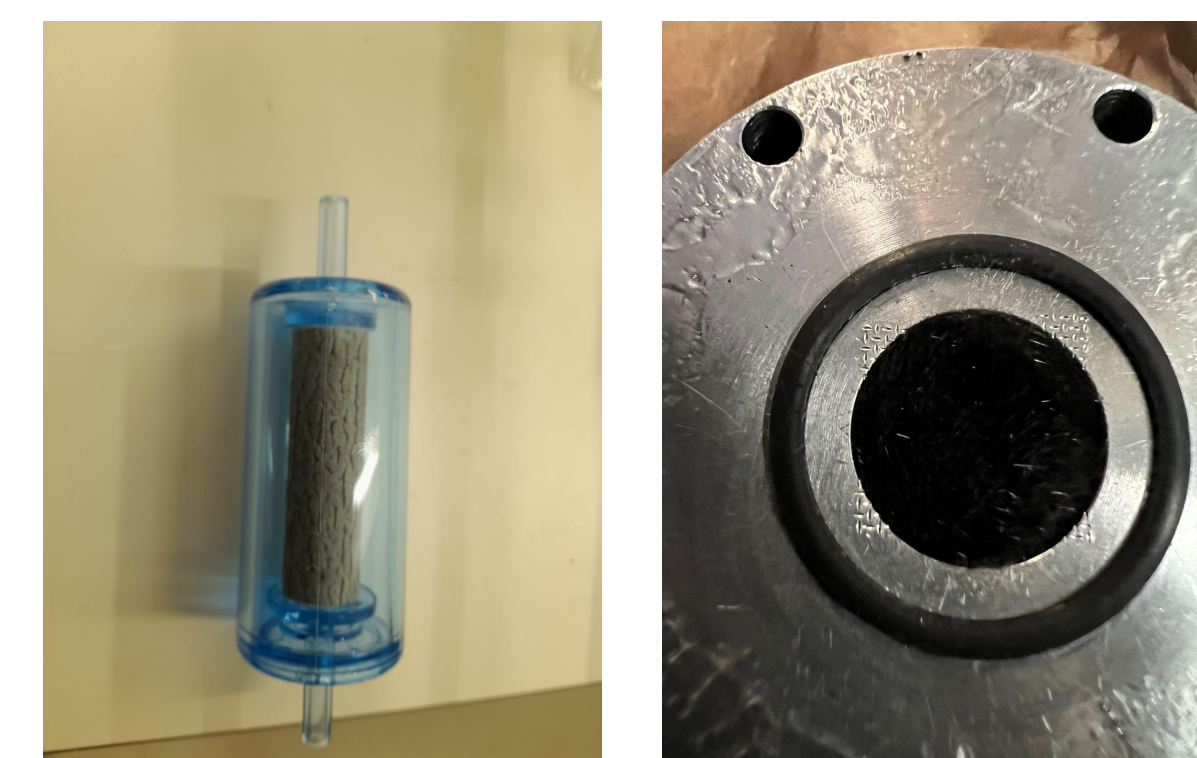
Figure 6: Smoke captured on the Teflon filter (left) and PAH filter (right).
