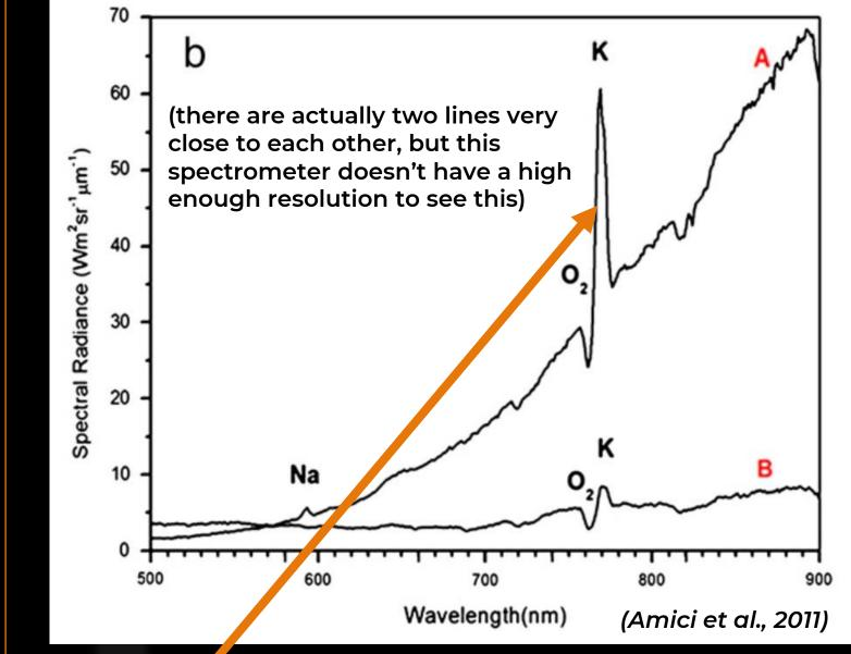
We measured a fire from the side using a hyperspectral imager. This imager is usually used from an aircraft. For each pixel it measures light at many wavelengths with very high resolution from the red to near infrared (indicated by the colour under the curve in the spectra below).
